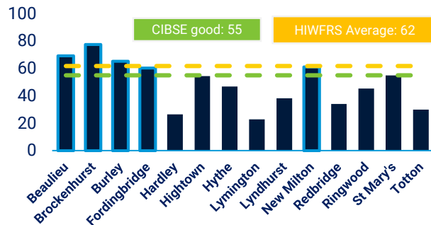
Electricity intensity (kWh/m 2 )
